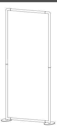
Assemble frame in numerical order, apply graphic pillowcase then attach bases #7 and 8.
